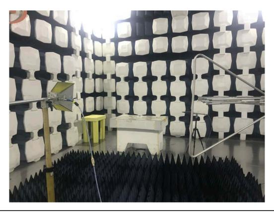
(2) Radiated spurious emission Test Setup(1GHz~18GHz)
