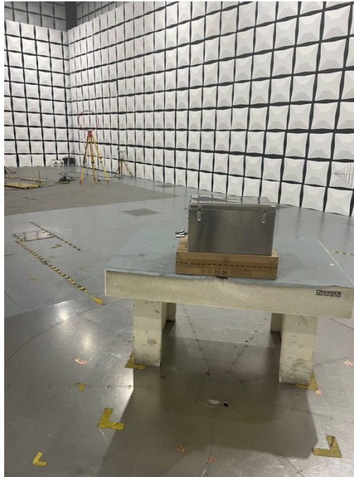
(2) Radiated spurious emission Test Setup(30MHz~1GHz)
