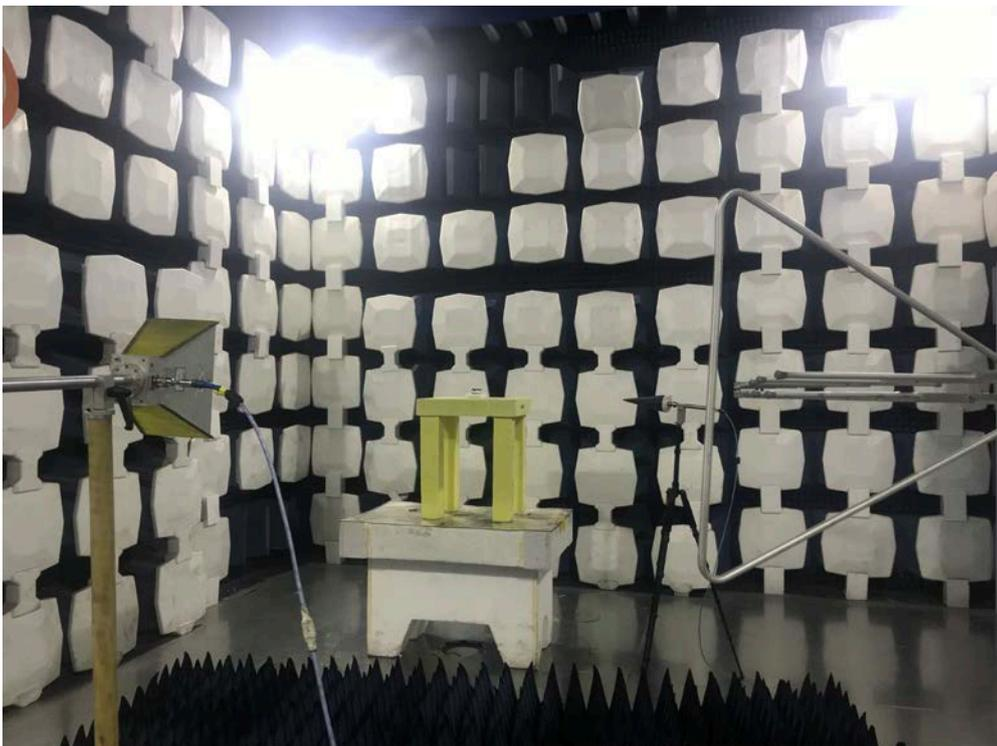
(3) Radiated spurious emission Test Setup(18GHz~26GHz)
