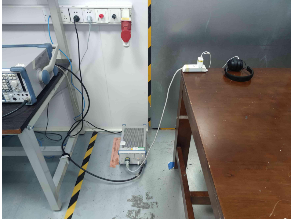
Conducted emissions at AC power line (150kHz-30MHz)
