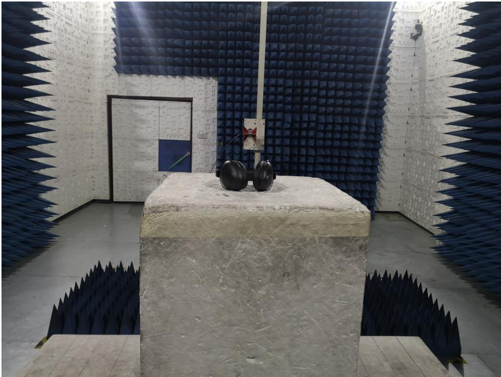
RADIATED EMISSION TEST SETUP ABOVE 1GHZ
