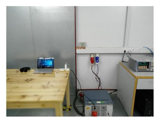
**RADIATED EMISSION TEST SETUP**
