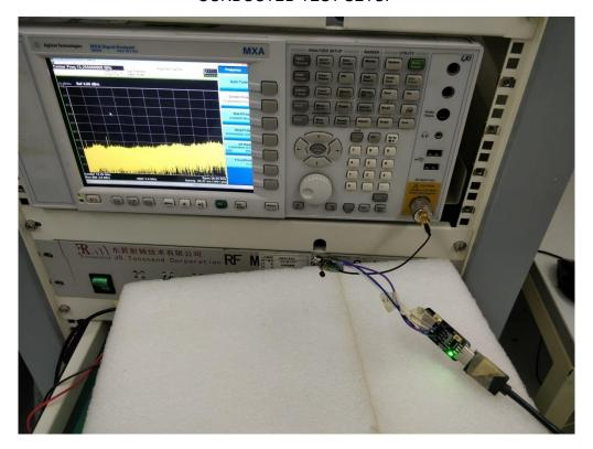
RADIATED SPURIOUS EMISSION TEST SETUP
