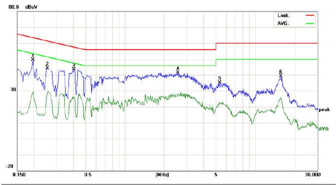
Site: Conduction Phase: L1 Temperature: 23.1 Limit: FCC Class B Conduction(QP) Power: Humidity: 54.7 %
