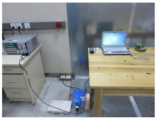
FCC RADIATED EMISSION TEST SETUP
