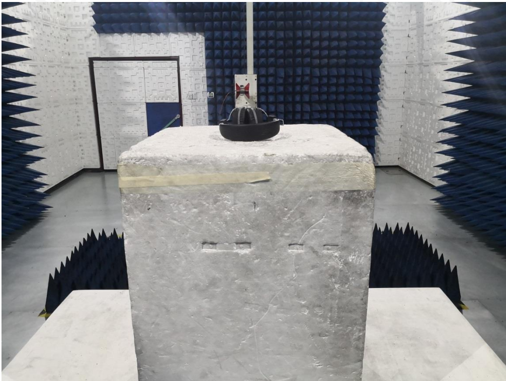
RADIATED EMISSION TEST SETUP ABOVE 1GHZ
