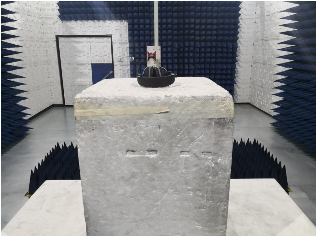
RADIATED EMISSION TEST SETUP ABOVE 1GHz
