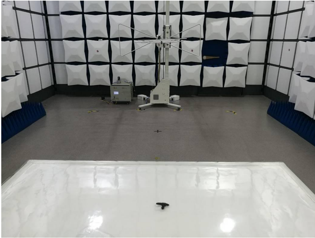
FCC RADIATED EMISSION TEST SETUP
