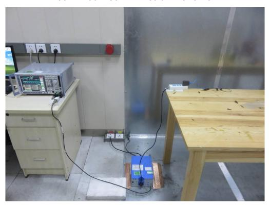
FCC RADIATED EMISSION TEST SETUP
