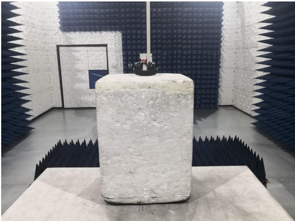
RADIATED EMISSION TEST SETUP ABOVE 1GHz
