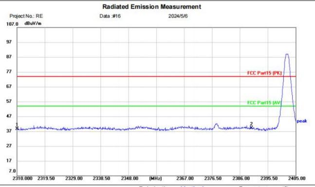
Site Polarization: Vertical Temperature: (C)
