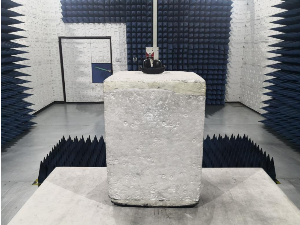
RADIATED EMISSION TEST SETUP ABOVE 1GHz
