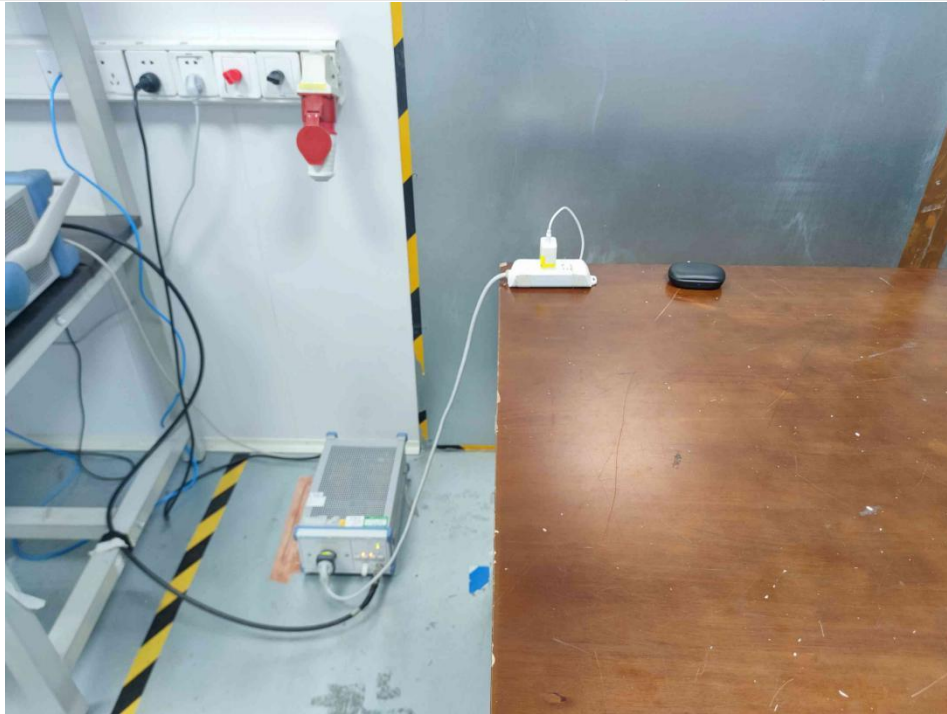
Conducted emissions at AC power line (150kHz-30MHz)
