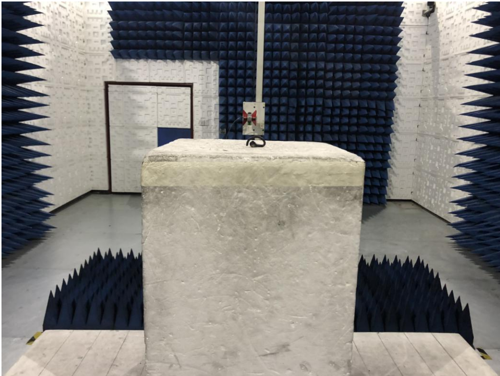
RADIATED EMISSION TEST SETUP ABOVE 1GHZ
