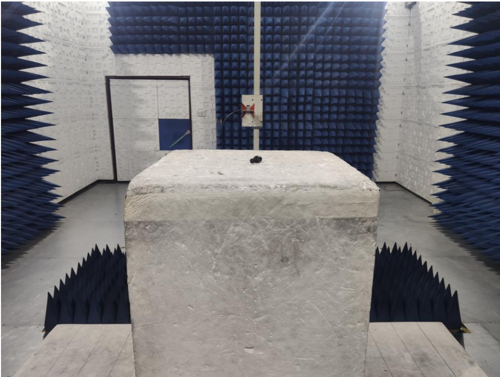
RADIATED EMISSION TEST SETUP ABOVE 1GHZ
