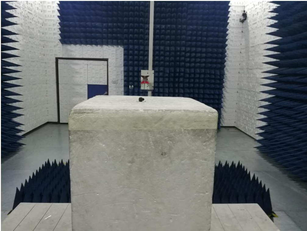
RADIATED EMISSION TEST SETUP ABOVE 1GHZ
