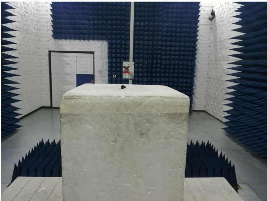
RADIATED EMISSION TEST SETUP ABOVE 1GHZ
