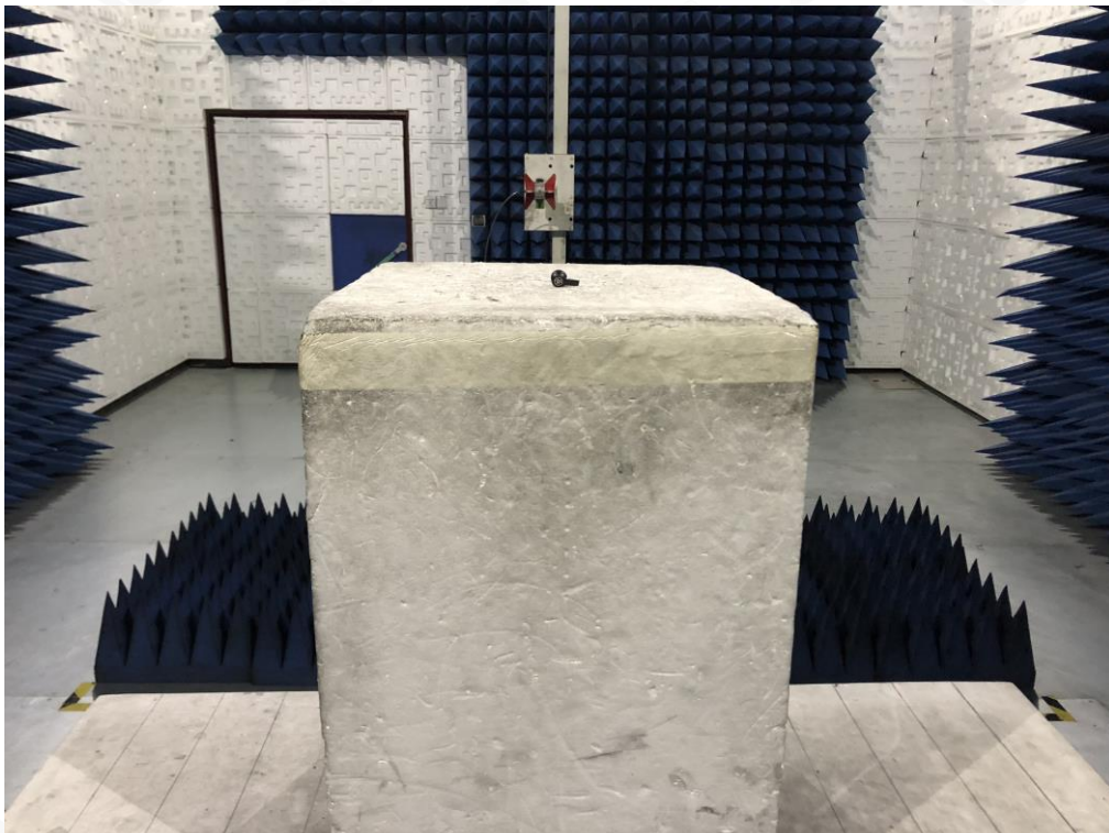
RADIATED EMISSION TEST SETUP ABOVE 1GHZ
