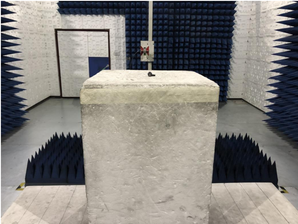
RADIATED EMISSION TEST SETUP ABOVE 1GHZ
