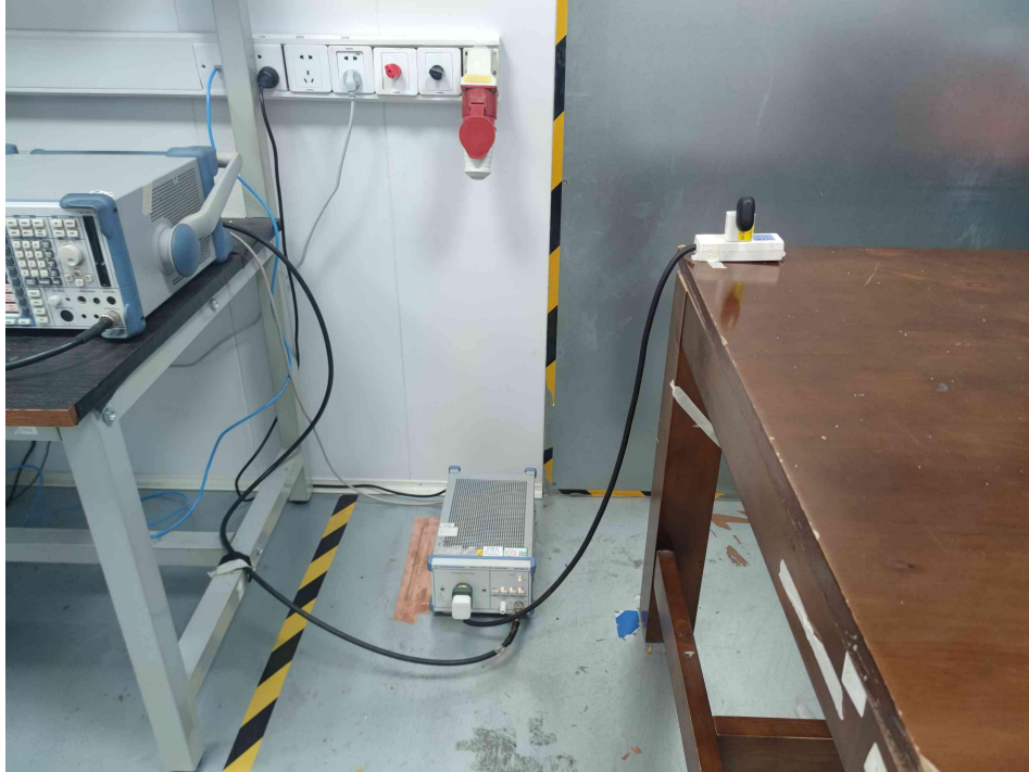
Conducted emissions at AC power line (150kHz-30MHz)
