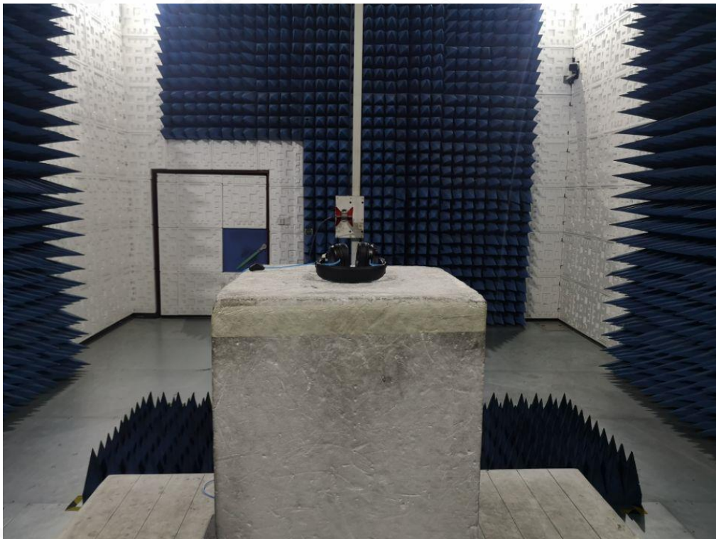
RADIATED EMISSION TEST SETUP ABOVE 1GHZ
