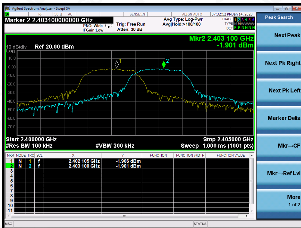
TEST PLOT FOR FREQUENCY SEPARATION
