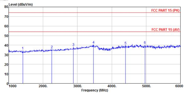
3m chamber FCC PART 15 (PK) 3m HORIZONTAL GTS201611000158 Site Condition
