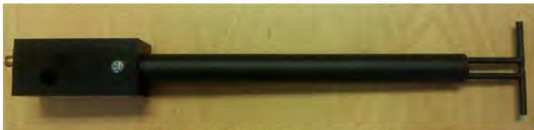
Figure 1 – MVG COMOSAR Validation Dipole
