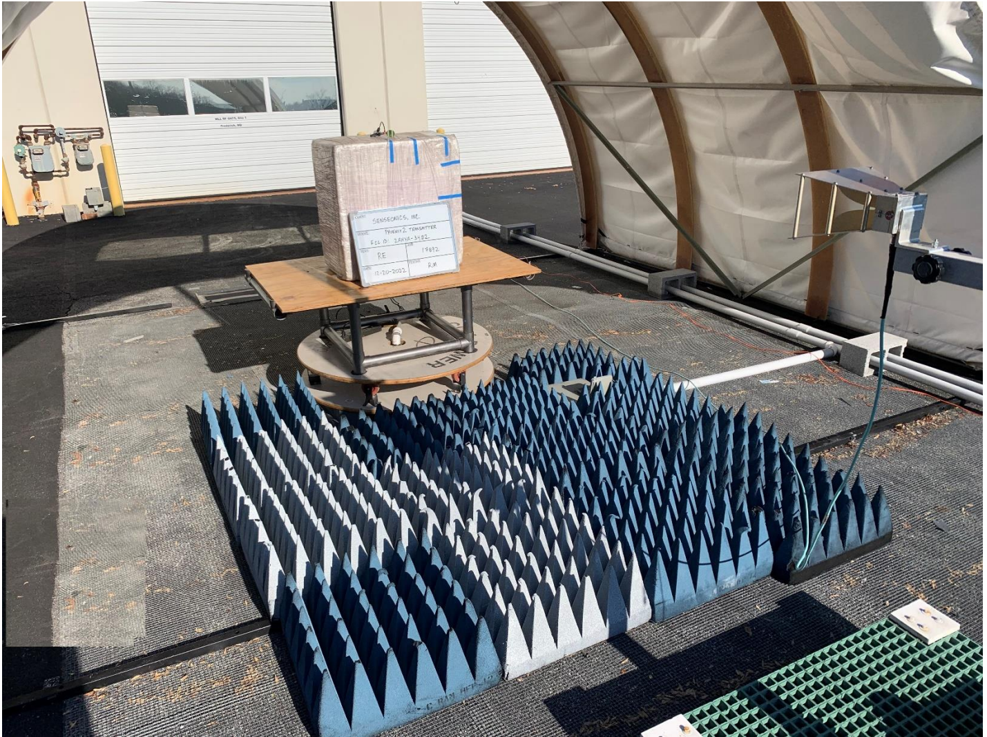
Radiated Emissions Font View, > 1GHz
