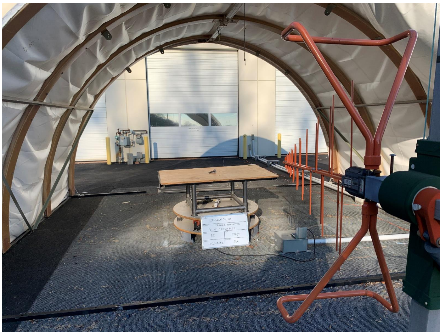
Radiated Emissions Font View, < 1GHz
