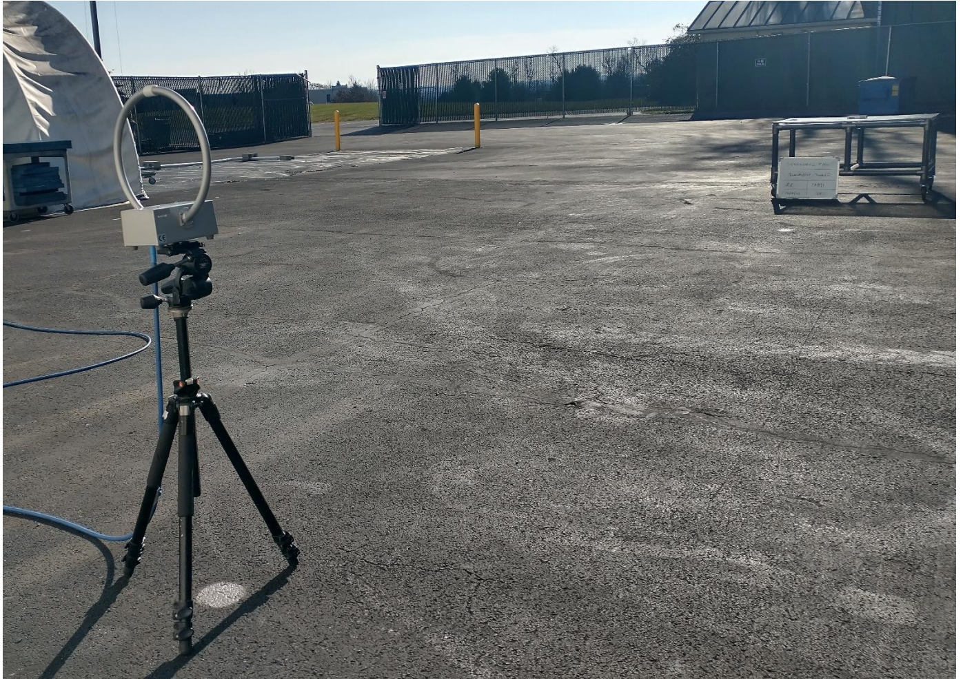
10-meter Radiated Emissions Test Setup, < 30MHz
