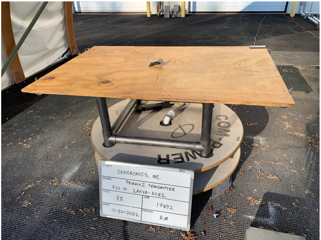
Radiated Emissions, < 1GHz
