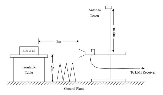
Frequency:9kHz-30MHz Frequency:30MHz-1GHz Frequency: Above 1GHz RBW=10KHz, RBW=120KHz, RBW=1MHz, VBW=3MHz(Peak), 10Hz(AV) VBW = 30KHzVBW=300KHz Sweep time= Auto Sweep time= Auto Sweep time= Auto Trace = max holdTrace = max holdTrace = max hold Detector function = peak Detector function = peak, QP Detector function = peak, AV
