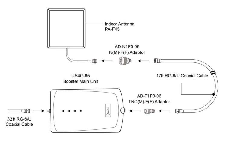
(Option) Connection of 11ft RG-6/U Extension Coaxial Cable
