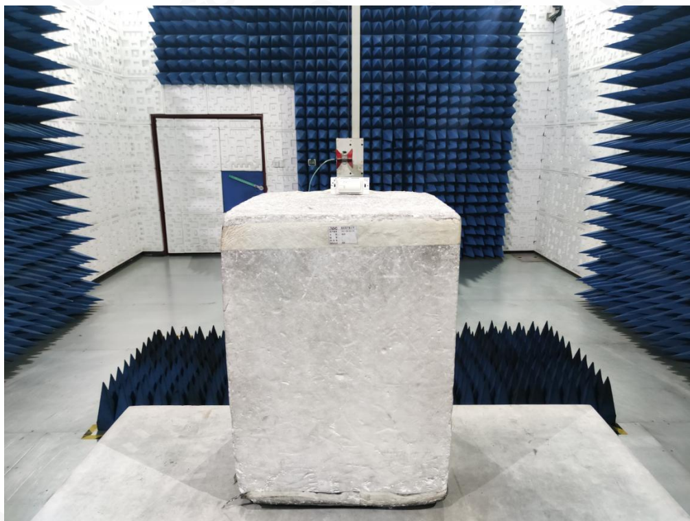
FCC RADIATED EMISSION TEST SETUP-ABOVE 1GHz
