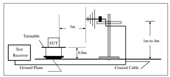
(b) For radiated emissions above 1000MHz
