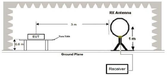
(2) Radiated Emission Test-Up Frequency 30MHz~1GHz
