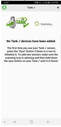
3. Press and hold SYNC button until sensor appears on app. (up to 10 seconds)
