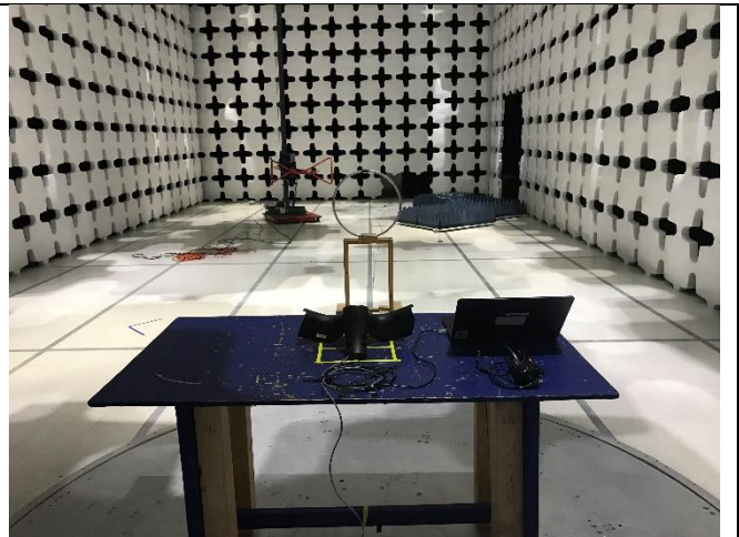
Radiated Emissions (<30MHz) – Rear View
