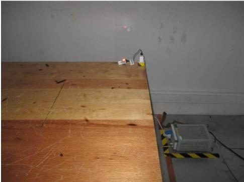
1.2 Radiated Spurious Emissions Test Setup
