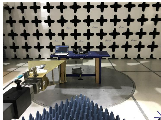
Radiated Emissions (>1GHz) – Front View
