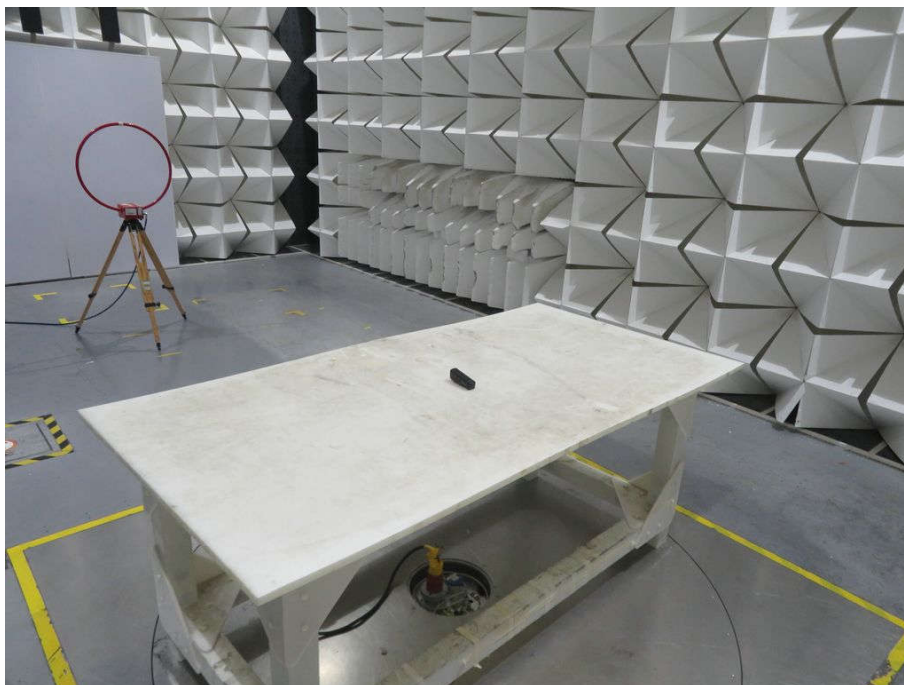
Radiated spurious emission Test Setup-1(Below 30MHz)
