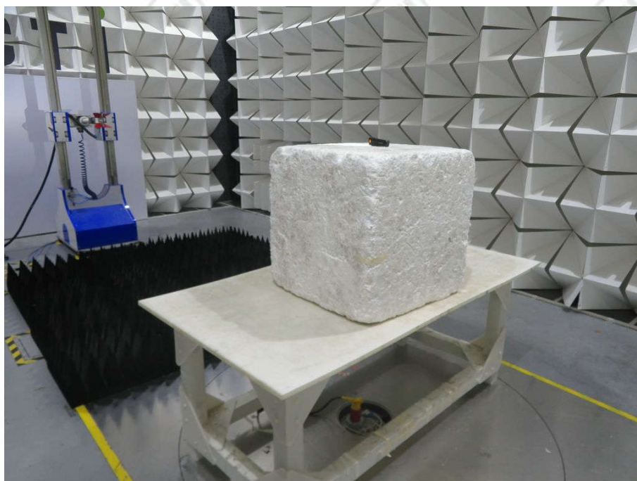
Radiated spurious emission Test Setup-3(Above 1GHz)
