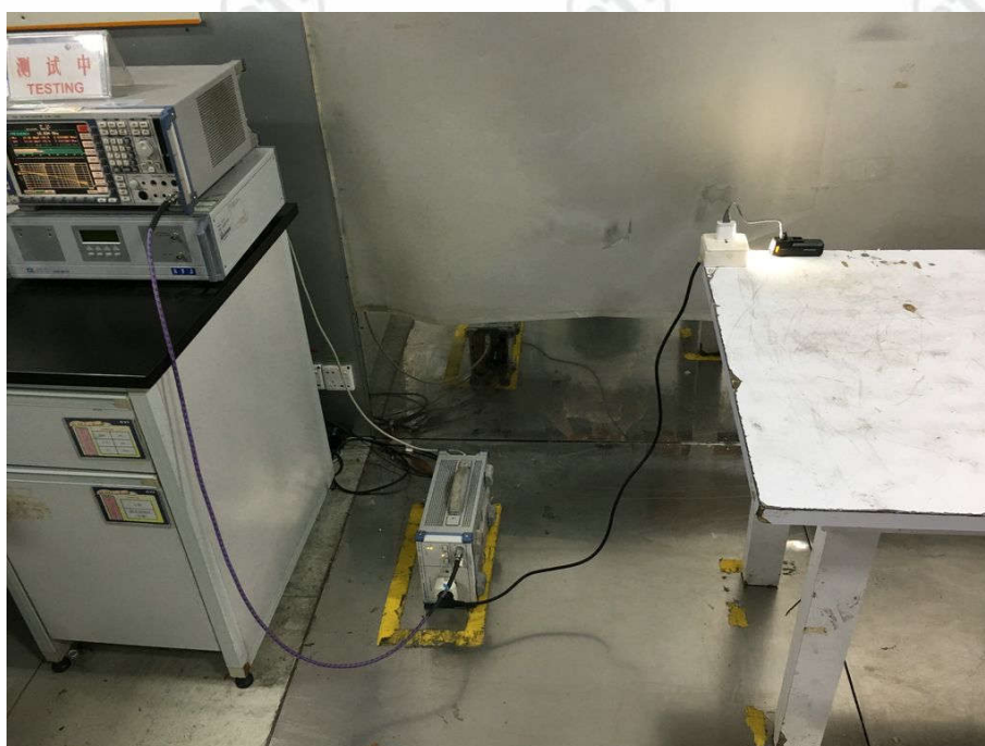
Conducted Emissions Test Setup
