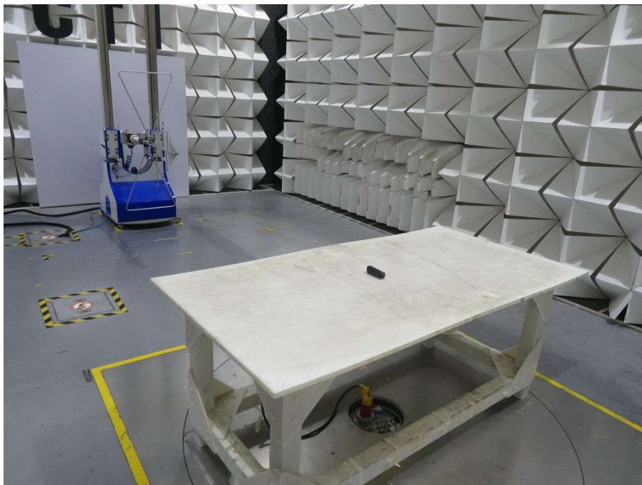
Radiated spurious emission Test Setup-2(Below 1GHz)
