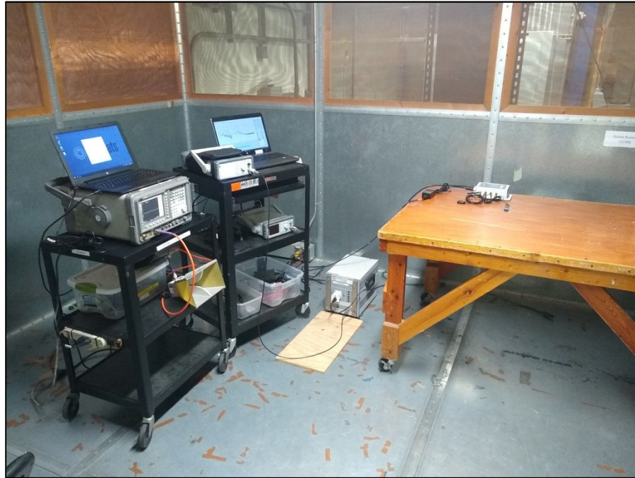
Photograph 5. Conducted Emissions Voltage, , Test Setup
