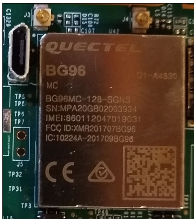
Photograph 4. Cellular Module (Quectel BG96)
