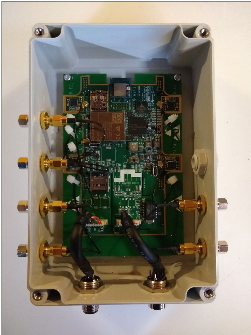
Photograph 1. EUT – Front Cover Removed
