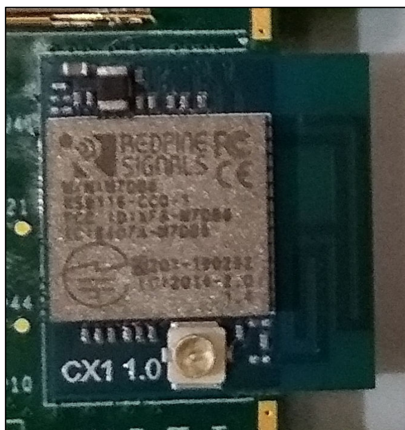
Photograph 5. WLAN Module (RedPine RS9116W-DB00-CC1)
