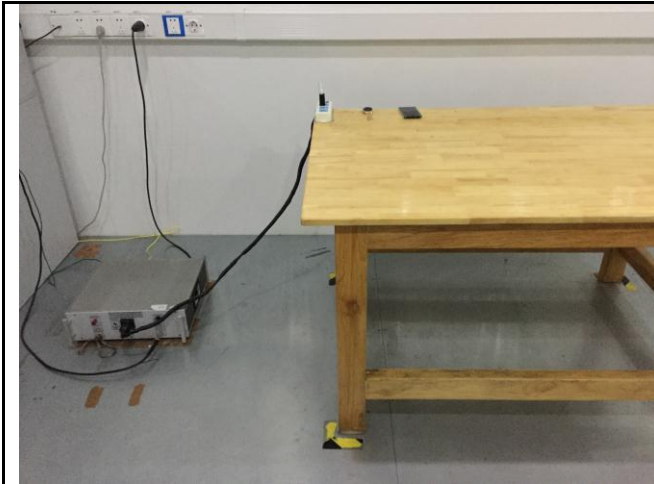
Conducted Emissions Test Setup Front View
