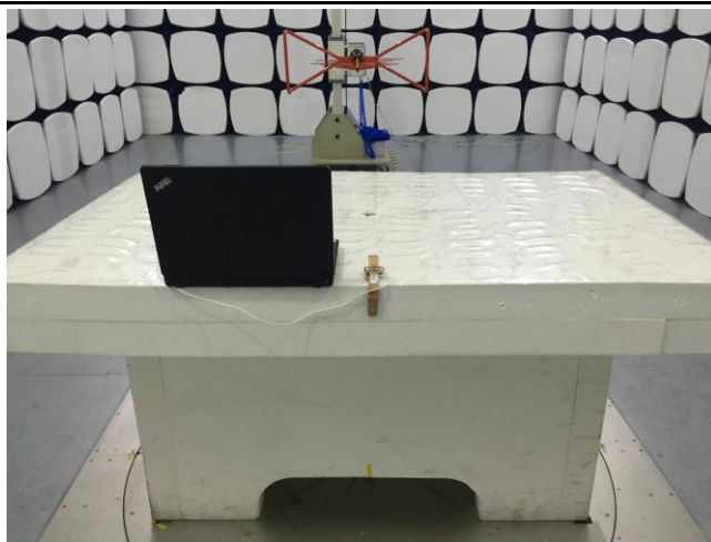
Conducted Emissions Test Setup Front View
