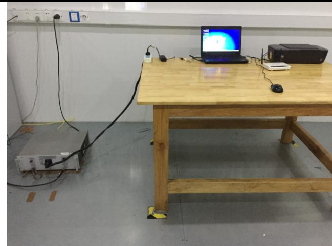
Conducted Emissions Test Setup – Front View
