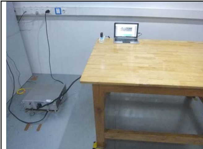
Conducted Emissions Test Setup Front View
