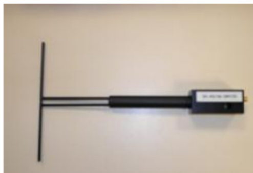
Figure 1 – Satimo COMOSAR Validation Dipole
