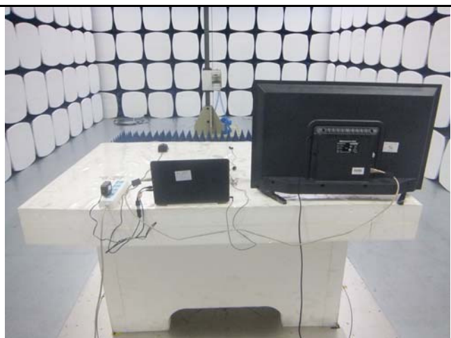
Radiated Emissions Test Setup Above 1GHz
