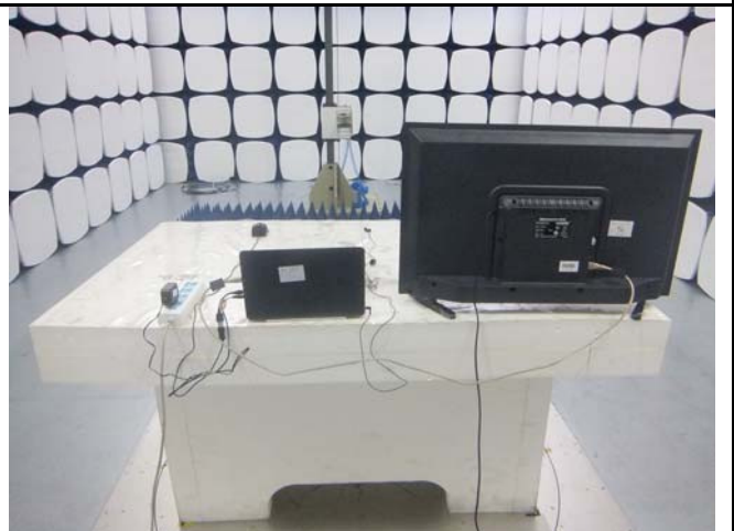
Radiated Emissions Test Setup Above 1GHz
