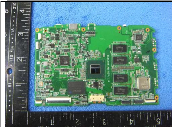
Mainboard with Shielding - Front View
