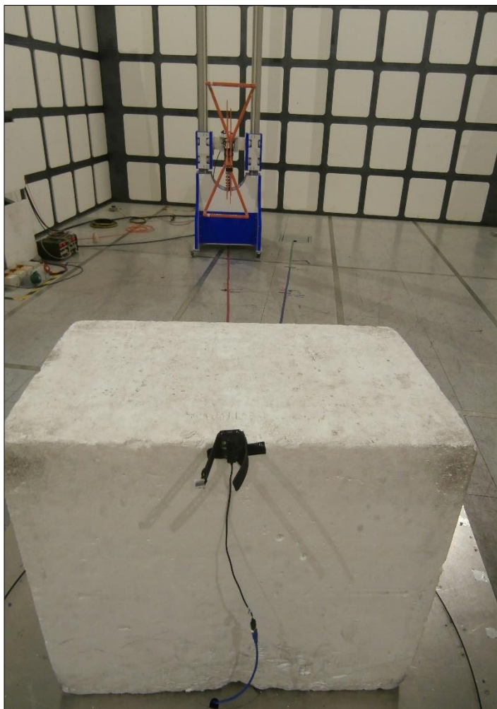
Figure 26 - Test Setup - 30 MHz to 1 GHz - Z Orientation
