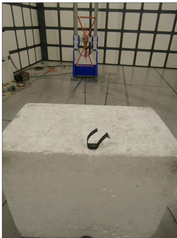
Figure 57 - Test Setup - 30 MHz to 1 GHz
