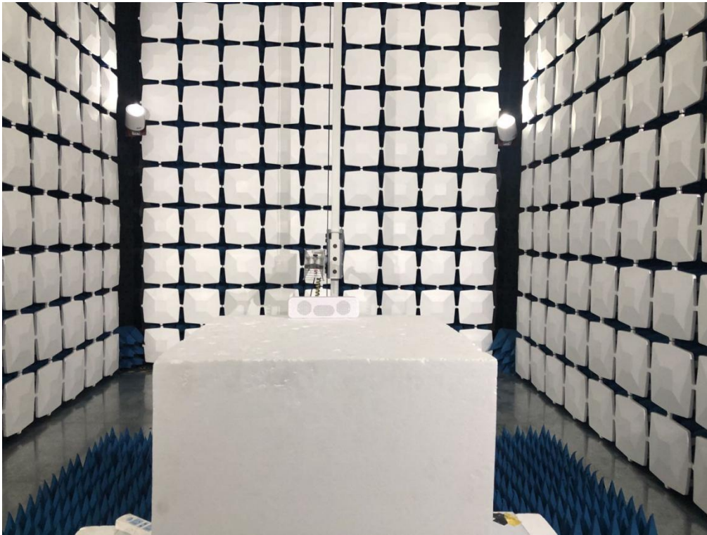
Above 1GHz for radiated emission test setup
