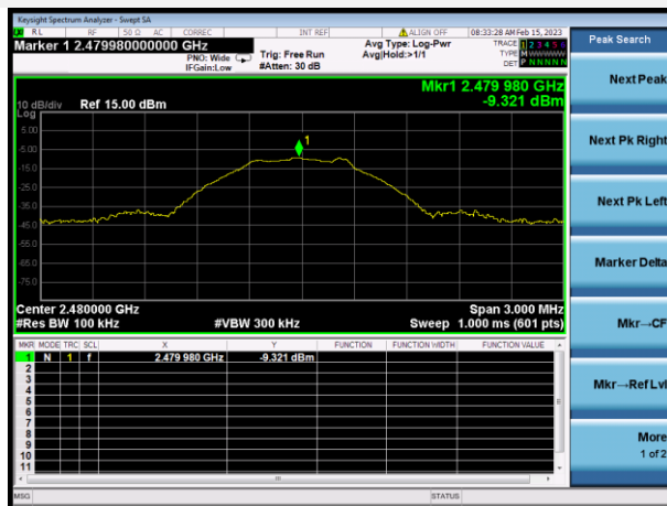
GFSK (BLE 1Mbps) HIGH CHANNEL, CARRIER LEVEL
